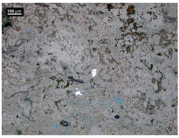
**Fig 17. Blue lead sulphide in the lump Blejeşti 1–2, near galena inclusions.** OM, bright field (S. Rovira). https://doi.org/10.1371/journal.pone.0214218.g017
