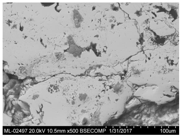
**Fig 20. Detail of the lead oxide layer (white) showing the grey inclusions of complex oxides containing Fe, Zn, Pb and Cu.** Blejeşti 1–1 sample. SEM image, backscattered electrons (S. Rovira).
