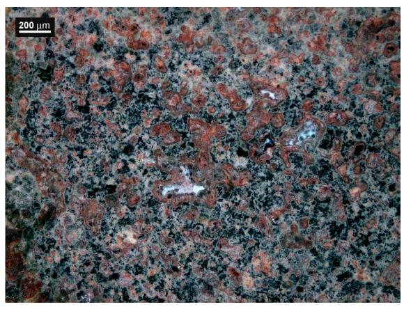
**Fig 23.** Appearance of the lump Blejeşti 1–2 core showing the colour diversity of its phases. The anglesite appears black, reddish, white and transparent crystalline. Palmierite is dispersed in clear crystalline form. OM image, Dark Field (S. Rovira).
