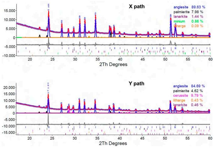
Fig 13. Diffraction patterns of the leaded lump Blejeşti 1-2 (S. Rovira).
