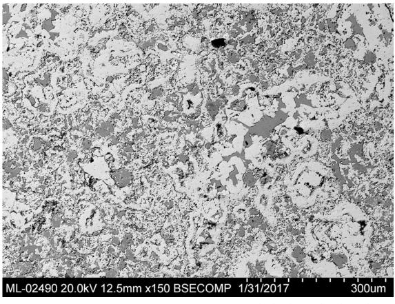
**Fig 14.** Aspect of the phase distribution in the core of the leaded lump Blejeşti 1–2. The white phase is anglesite, the grey phase is palmierite. SEM image, backscattered electrons (S. Rovira).
