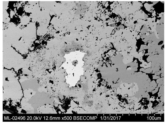
Fig 16. Lead sulphide inclusion in the lump Blejeşti 1–2. 1 galena, 2 litharge, 3 anglesite. SEM image, backscattered electrons (S. Rovira).
