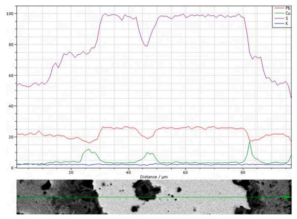
**Fig 18.** Line scan for the relative concentration of S, Pb, Cu and K in the inclusion of galena and its surroundings in Blejeşti 1–2. Explanation in the text. SEM analysis (S. Rovira).
