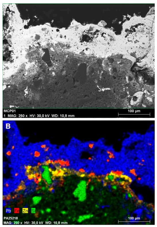
**Fig 21.** Section of the Blejeşti 1–1 sample (A) and distribution map of the elements Pb, Fe, Zn and Si (B). SEM image, backscattered electrons (S. Rovira).
