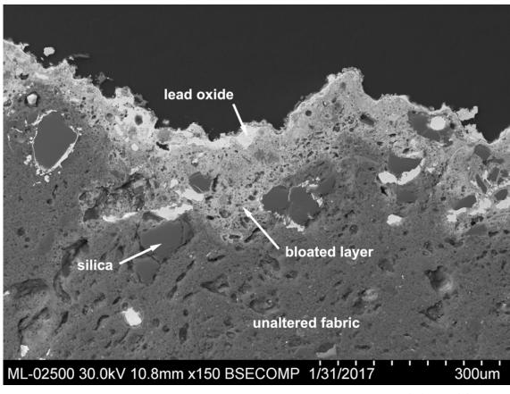
Fig 19. Section of the Blejeşti 1–1 piece showing the location of the main structural phases. SEM image, backscattered electrons (S. Rovira).
