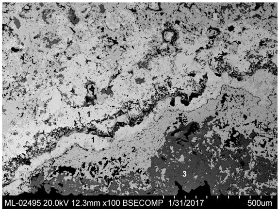
Fig 15. Part of the lump Blejeşti 1–2 corresponding to the superficial crust. 1 lead oxide (litharge), 2 lead sulphate (anglesite), 3 potassium-lead sulphate (palmierite). SEM image, backscattered electrons (S. Rovira).
